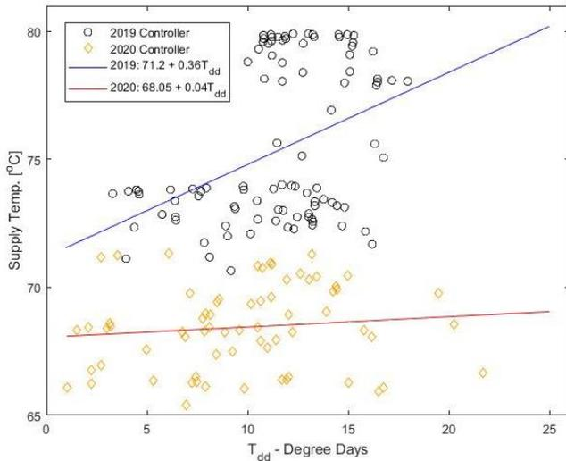
In HEAT 4.0 the state-of-the-art temperature optimization has been implemented in Brønderslev, Denmark. The results have been a lower supply temperature. The supply temperature with the new controller is 4-7°C lower. In Svebølle-Viskinge, a similar system has been installed. Here the temperature was lowered with approx. 12°C.
